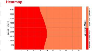
Torque [Nm] Note: Assuming 25°C ambient temperature and 10 m/s airflow.
