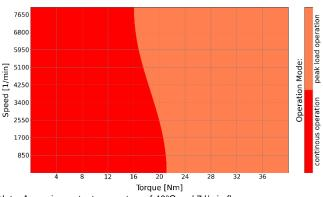
Note: Assuming water temperature of 40°C and 7 l/min flow.
