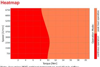
Note: Assuming 25°C ambient temperature and 10 m/s airflow.
