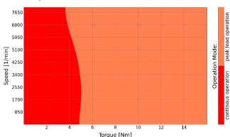
Note: Assuming 25°C ambient temperature and 10 m/s airflow.
