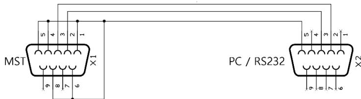
Figure 6: RS232 Connection without analog control
